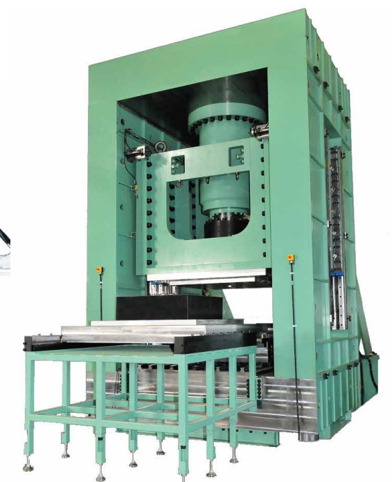
免震ゴム用二軸試験機 Double axis testing machine for seismic isolation rubber bearings
